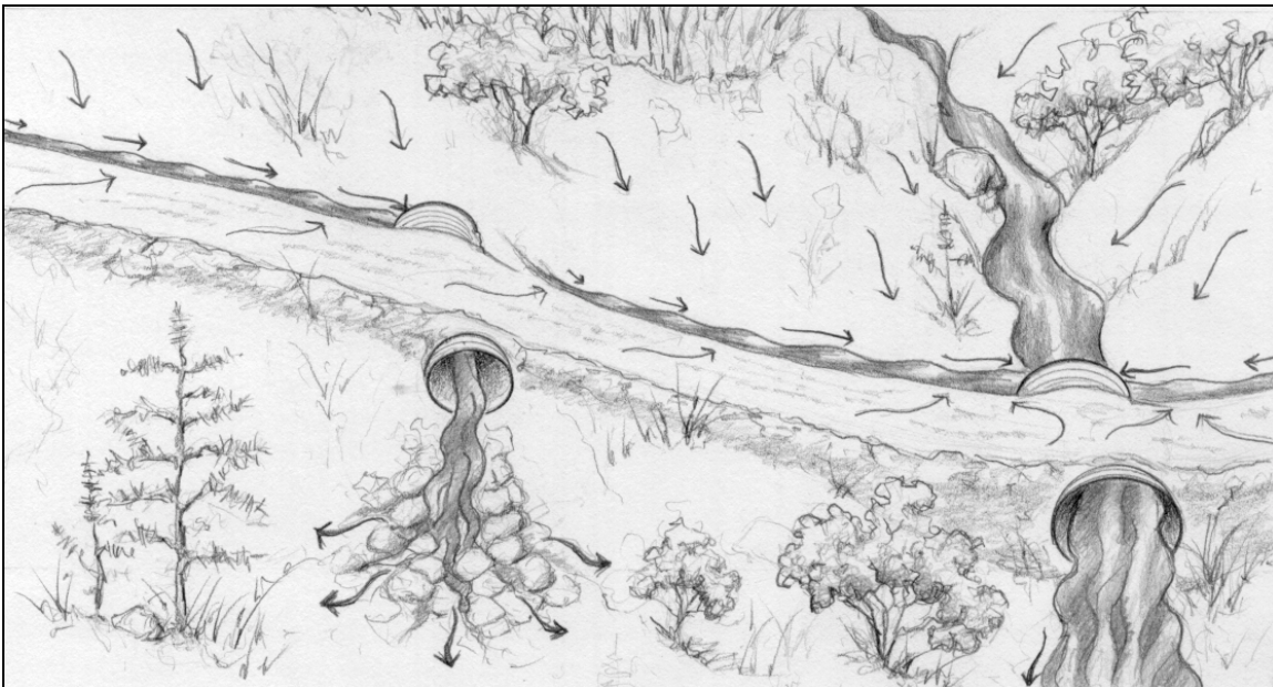
Figure 5-9. Road Drainage Issues Affecting Stream Channel Stability
