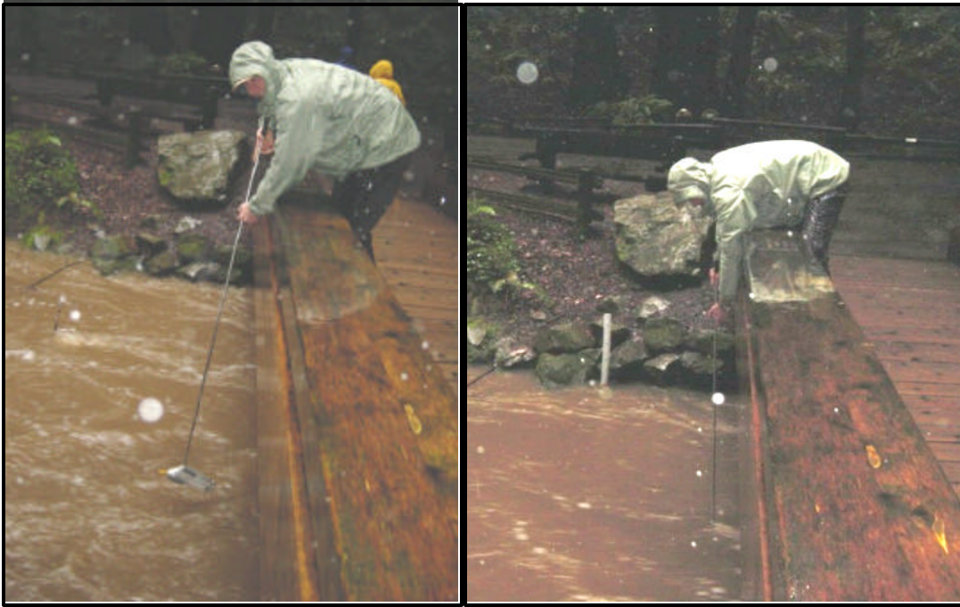
Figures 2 and 3. Suspended sediment sampling. Lowering and raising a DH-48 sampler into the flow across the channel and a temporary gage on left bank.
