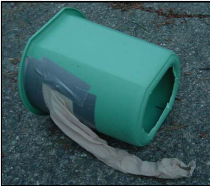
Figure 4. Hess-like sampler used to sample aquatic insects in Redwood Creek. A plastic garbage can with a 0.5 ft opening and a nylon stocking to catch the sample.
