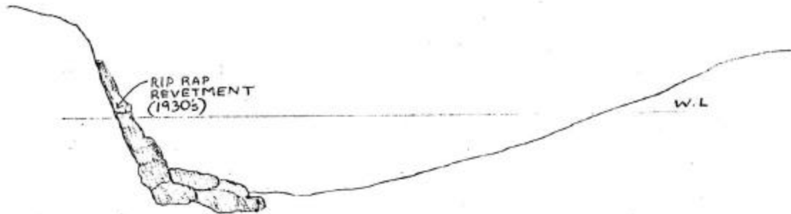
Figure 13. Cross section diagram of CCC rock revetment construction showing the bank protected along the toe and into the channel bed (From Howell and Milestone, 1981).
