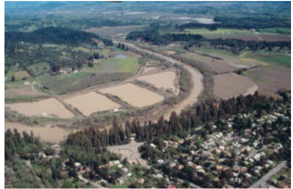
Sonoma County Water Agency Mirabel infiltration ponds and water diversion facilities along the Russian River
