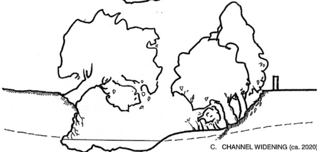
Figure 16. Conceptual representation of natural geomorphic recovery of entrenched stream channels showing pre-entrenchment condition, entrenched condition with confined active channel width and no gravel bar or floodplain formation, and recovered channel with increased active channel width, bar and floodplain formation, and increased near-channel riparian forest.
