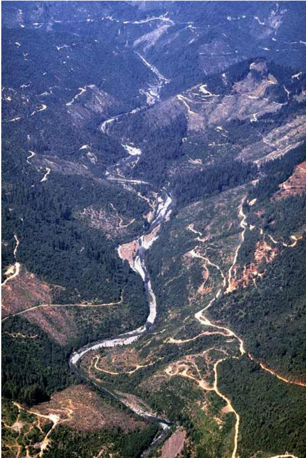
Figure 6. Inner gorge of Blue Creek in 1990 with clear cuts adjacent to the stream and a wide gravel bar signifying an over-supply of sediment from logging, landslides and failed roads.
