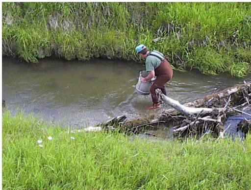
Using a Hess sampler to collect macroinvertebrates at site # TC1a
