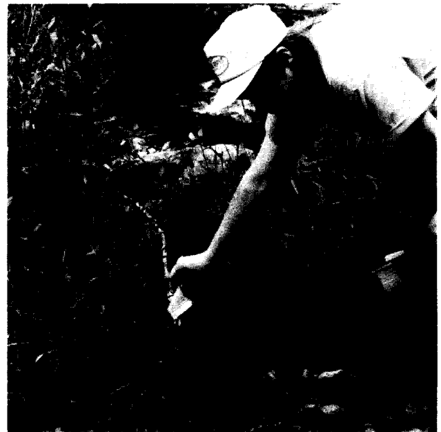
Figure 48. - Placing a pin flag at a change in vegetation.
